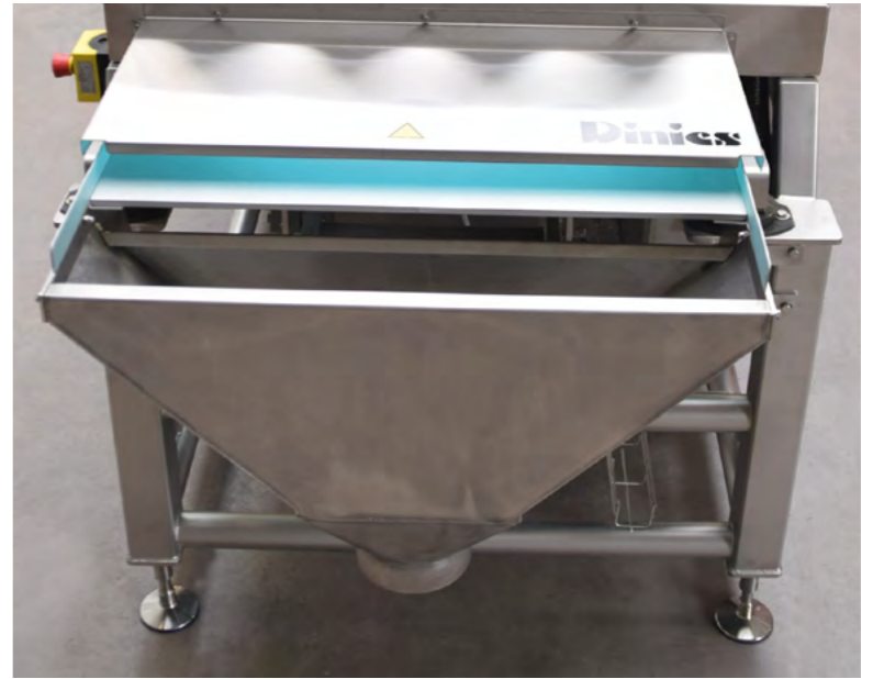
Filling funnel LxWxH 498x994x521mm
