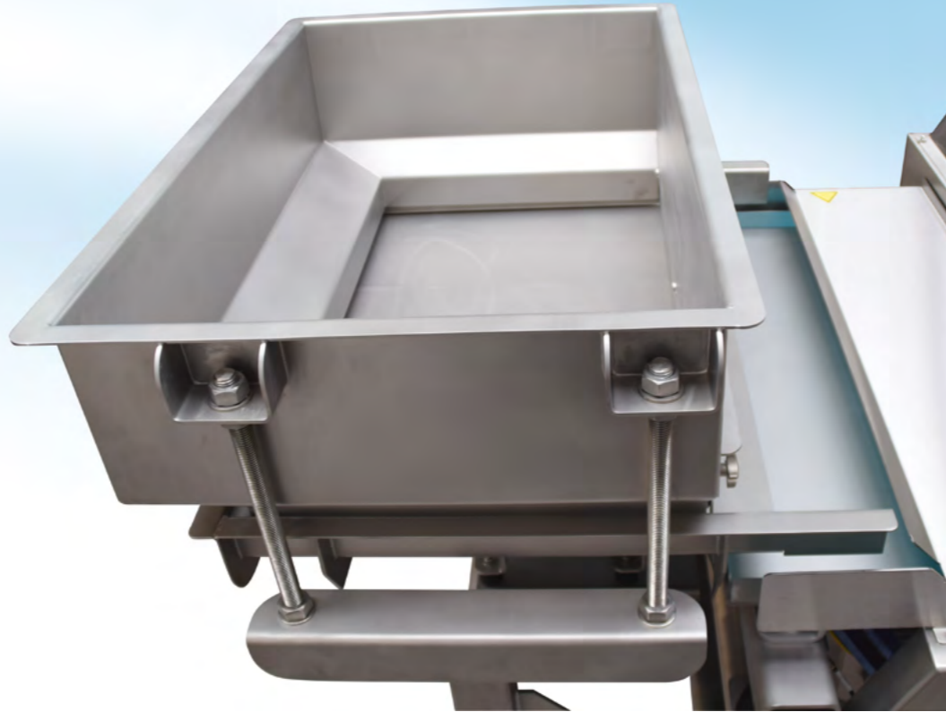
Silo hopper LxWxH 760x1060x1092mm
